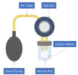
The **Hand Pump** provides positive air pressure.
